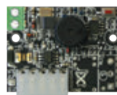
ACG9448 CARD to manage RADIO NUMERIC CODER and SUN remotes 1CH 433MHz - 125 codes from 4 to 9 digits - Only for the control panel of SLIDER
