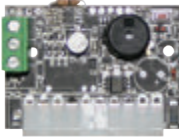
ACG9438 DECODER CARD for RFID READER It manages 125 RFID transponders Only for the control panel of SLIDER
